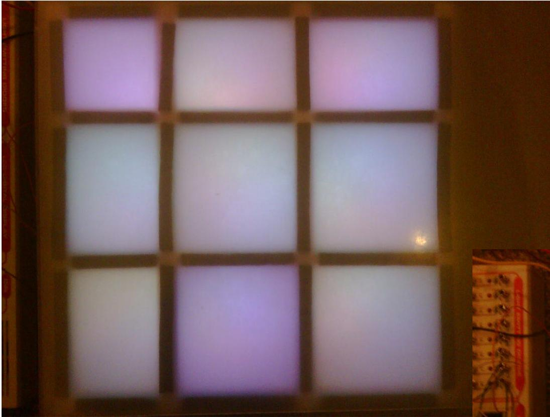
We first built a 3x3-cell test mini-floor, to experiment with different sized cells, test the strength of the acrylic, experiment with different sensors, and to test the electronics (including the shift-registers etc) on a small scale
